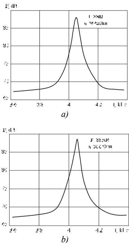
Fig. 4. AFC of piezoelectric transducers shown in the scheme: a) Fig. 3, a; b) Fig. 3, b
