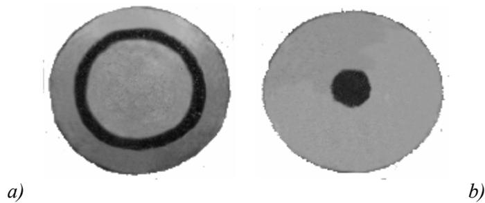
Fig. 2. Chladni figures for bending (a) and radial (b) oscillations of monomorph disk piezoelement
