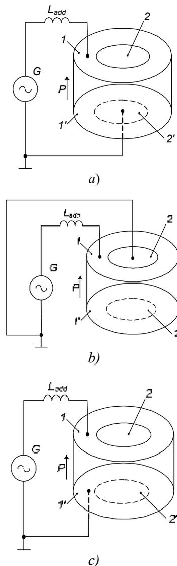
Fig. 5. Schemes of piezoelement connection with additional inductance:
