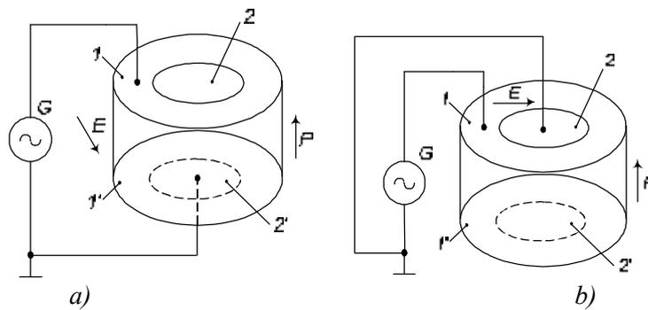
Fig. 3. Schemes of piezoelements connection: a)  $\alpha \approx 87^\circ$ , the electrodes 1 and 2' have coplanar location; b)  $\alpha = 90^\circ$ , the electrodes 1 and 2 have planar location
