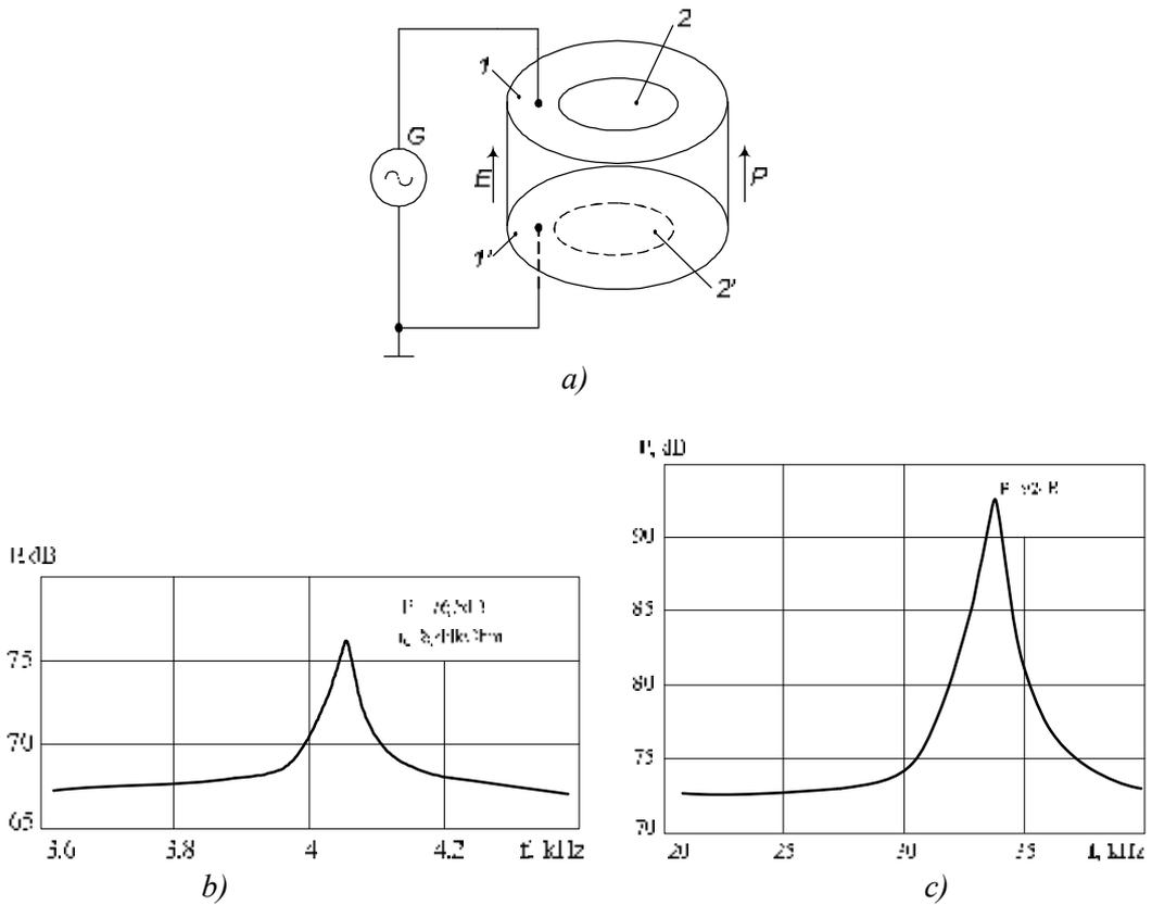
Fig. 1. Connection scheme (a), sound pressure amplitude-frequency characteristic at low-frequency (b) and high frequency (c) areas of monomorph piezoelectric element  $\varnothing 66 \times 3$  mm
